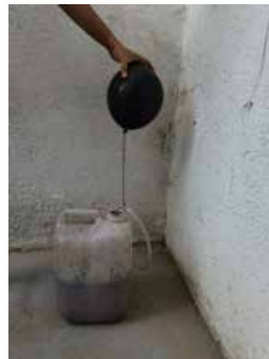
Fig. 5: Sufficient amount of Biogas generated at Day 35.
