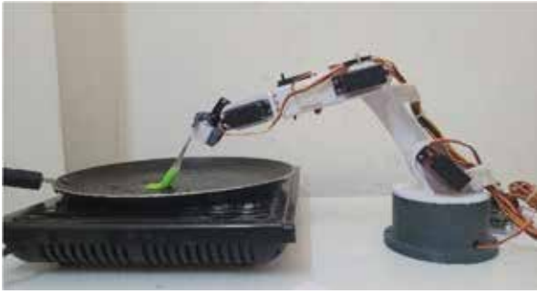
Fig. 5 (b): Robo applying oil on pan
