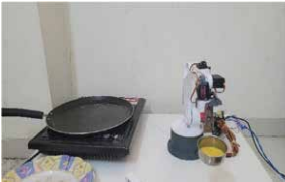
Fig. 5 (c): Robo picking up the egg batter
