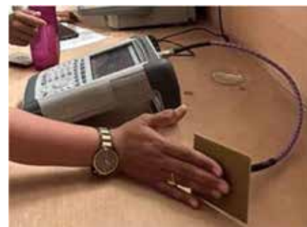
Fig. 9. Antenna resonating at 2.1GHz with return loss -17.5dB
