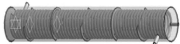
Figure 6: The Shell and Coil Heat Exchanger was modeled using CAD [9]
