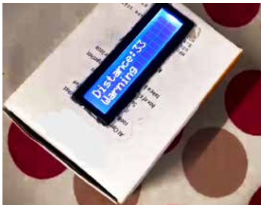
Fig. 4: LCD Display with reading (in cm) and a warning message
