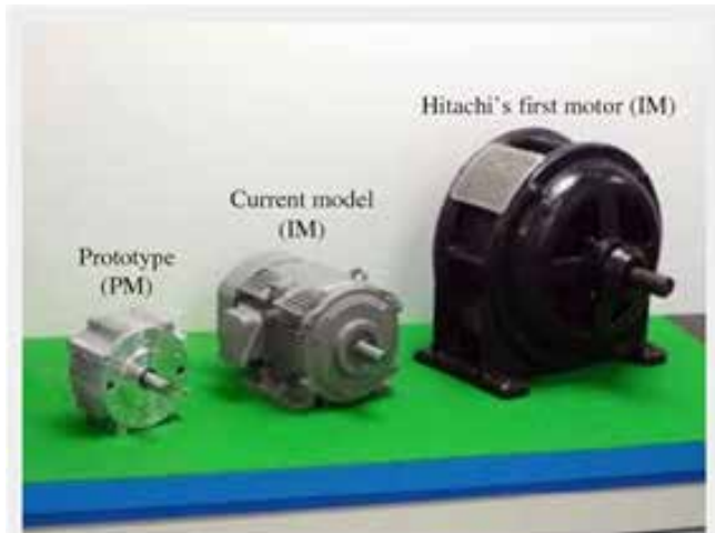
Fig. 6. Comparison of original 5-HP motor, current production model and new prototype [10]
