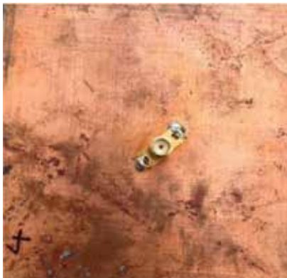
Fig 6. Coaxial Feedline (Bottom View)
