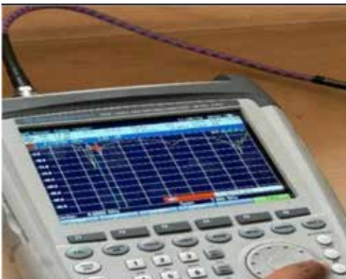
Fig. 11. Antenna not Resonating at 2.4 GHz
