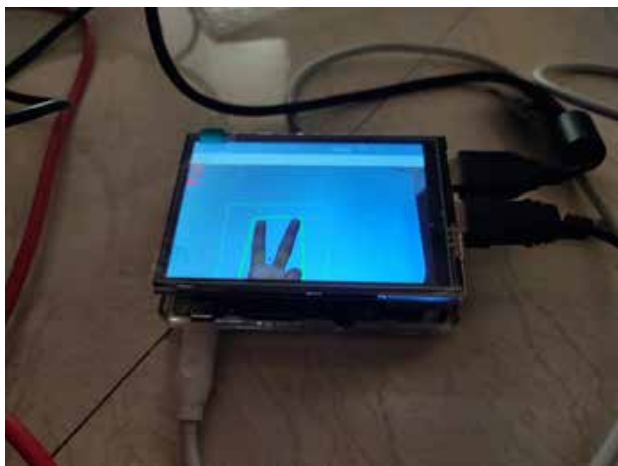
Fig. 6. Hardware Setup with Raspberry Pi and a HDMI display
