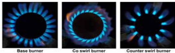
Figure 5: Flame shapes of (i) a no-swirl burner ( \theta = 0^\circ ), (ii) a Co- axial burner( \theta = 30^\circ ), and (iii) a Reverse-flow burner ( \theta = 30^\circ )[23]
