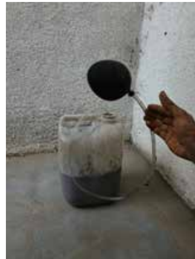
Fig. 4: Noticeable amount of biogas finally observed at Day 20
