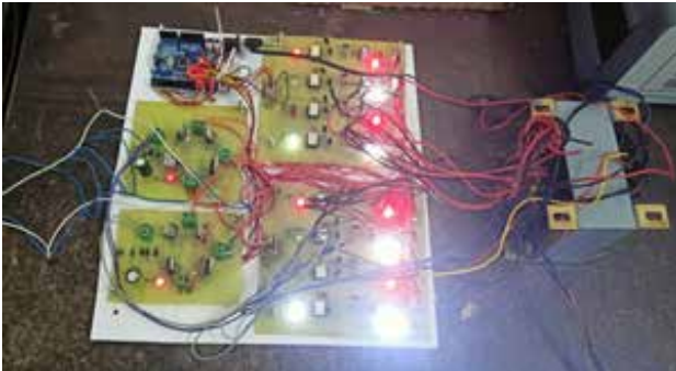
Fig. 4. Hardware Image of Proposed 7 Level CHBI
